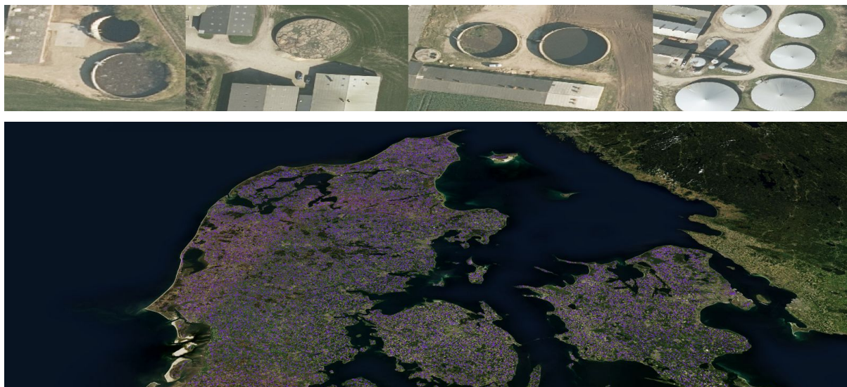
Figure 2. Slurry tanks detection over the whole country of Denmark (pink disks representing the farms).
