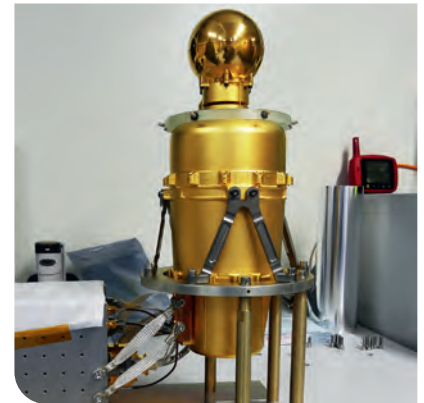
PFM of the NIM spectrometer of the PEP experiment on the ESA JUICE mission. Electronic box is on the left, sensor is in the middle.
